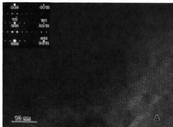
Fig. 2. Low-magnification electron-microscopy structure image of an \text{Sc}_2\text{S}_3 crystal. Inset at top left is the corresponding, indexed diffraction pattern: zone axis [\bar{1}10]_1 . The larger numbers (below a reflection) correspond to the \text{Sc}_2\text{S}_3 orthorhombic cell (1); the smaller numbers (above) correspond to the \text{NaCl} -type subcell.
